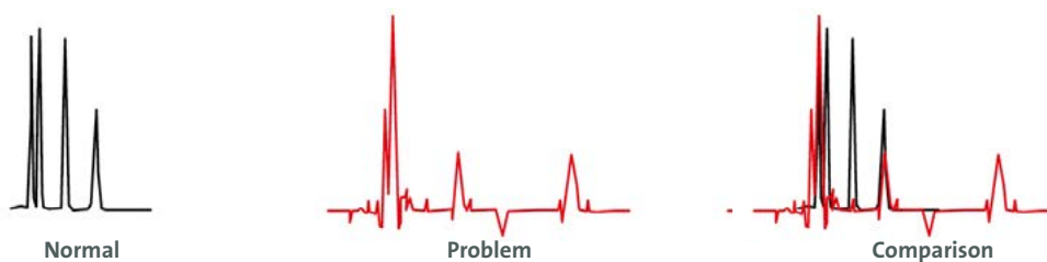
Figure 9: Chromatogram showing negative peaks.
