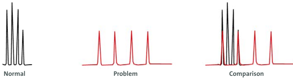
Figure 4: Illustrated chromatogram showing variable retention times.
